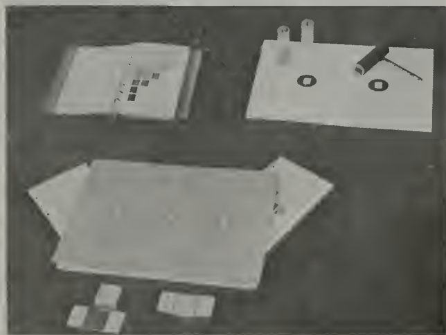
FIGURE 5. A triple-aperture shield with sample aperture in center and apertures for Munsell standards on each side.
